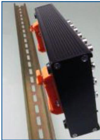
*With the optional DIN rail mounting kit (BNC DIN RAIL KIT), you can mount the DT9826 BNC model to a standard DIN rail.*
